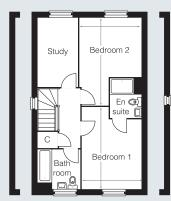
Plot 26 does not include windows to the hall and stairway as shown. Plot 26 includes windows to the w/c and ensuite as shown. Plots 26 & 34 are handed.
